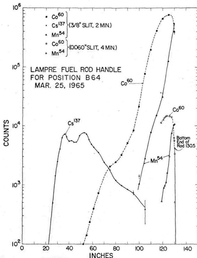
Fig. 10. Fission Product (and neutron induced) Radioactivity on a Typical Fuel Capsule Handle from LAMPRE. (The top of the handle is at the zero inch position; normal level of the sodium coolant was at approximately the 25 in. position.)
