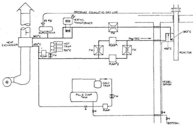
Fig. 6. Schematic Diagram of the Single-loop LAMPRE Coolant System.
