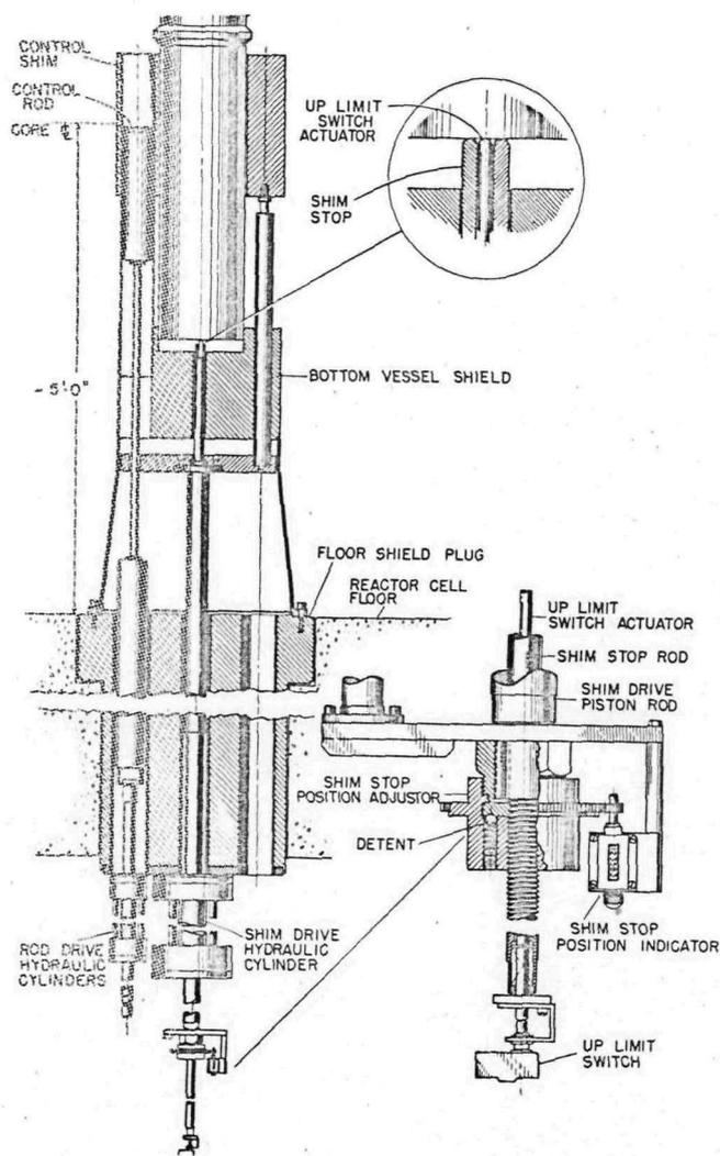
Fig. 5. LAMPRE Control Elements and Associated Hydraulic Cylinders for Actuation.
