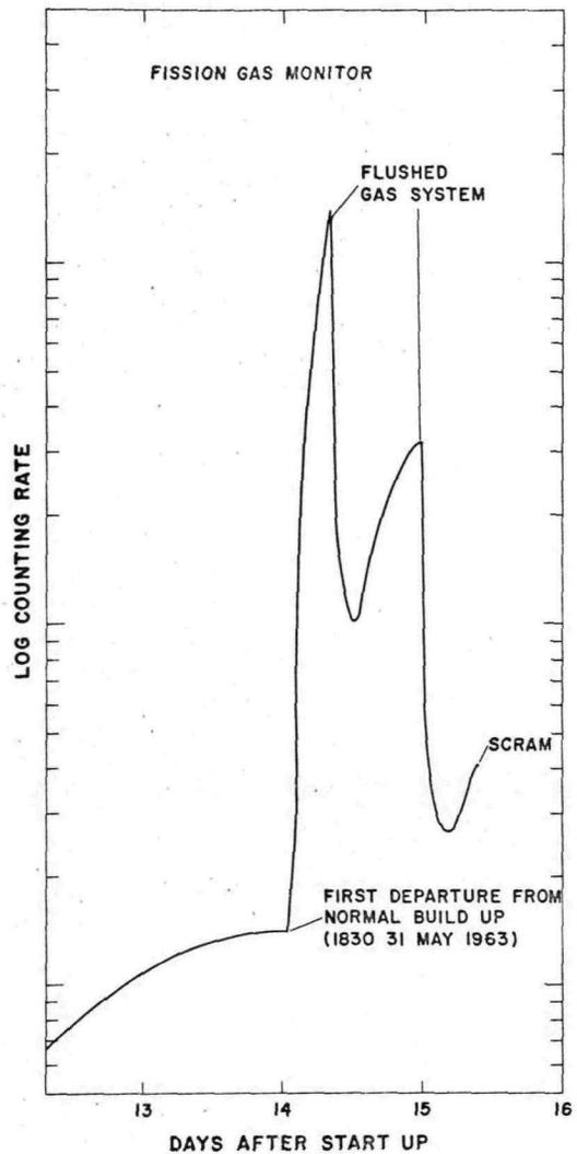
Fig. 9. Response of the LAMPRE Fission Product Monitor to Release of Fission Products in the Reactor Core.
