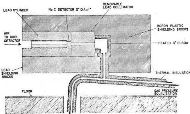
Fig. 8. Fission Product Detector on the LAMPRE Cover Gas System.
