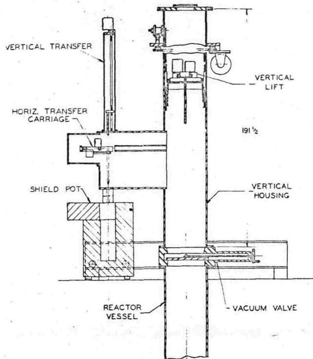
Fig. 11. LAMPRE Fuel Transfer Machine.
