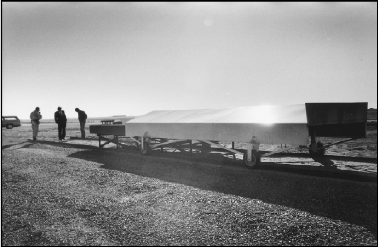
Burn trays are used to incinerate high explosive charges and debris from high explosive packaging on the grounds of the Pantex plant. Modern plastic-bonded high explosives will burn safely without detonating. Pantex was a conventional Army munitions plant before it began assembling nuclear weapons in 1951. Pantex Plant, Amarillo, Texas. November 18, 1993.
