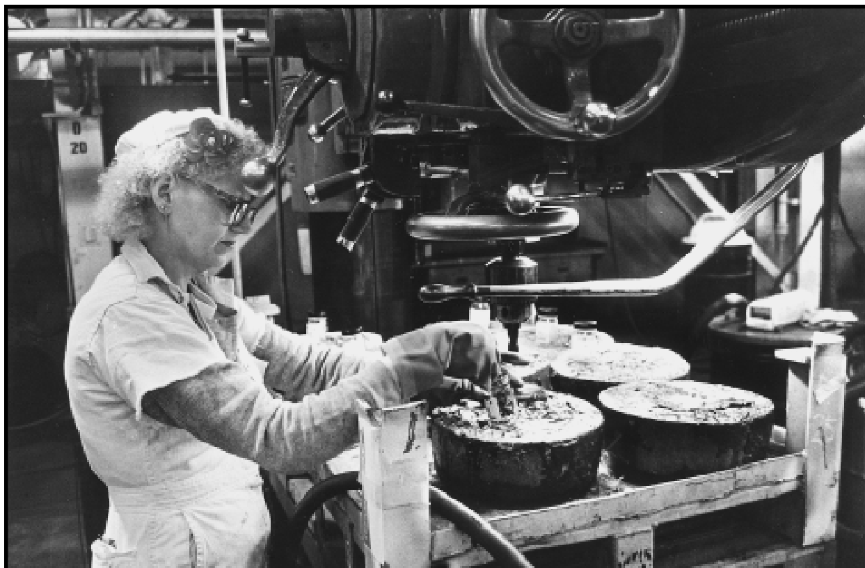
Sampling the Derby. A Fernald metals worker collects metal shavings from a new uranium derby. She will send them to an onsite laboratory which confirms the isotopic content and purity of the metal. Plant 5, Metals Production Plant, Feed Materials Production Center, Fernald, Ohio. December 17, 1985.
