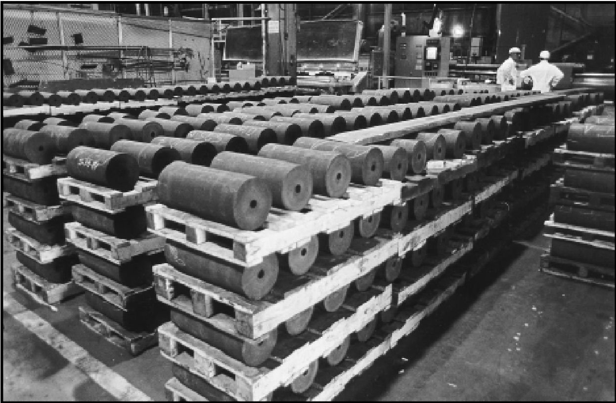
Depleted uranium metal billets were once an essential element in the production of weapons-grade plutonium. Today, billets like these are one of the Department of Energy's many types of materials in inventory. Each billet weighs about 1,100 pounds. Reactive Metals, Inc., Ashtabula, Ohio. June 19, 1984.
