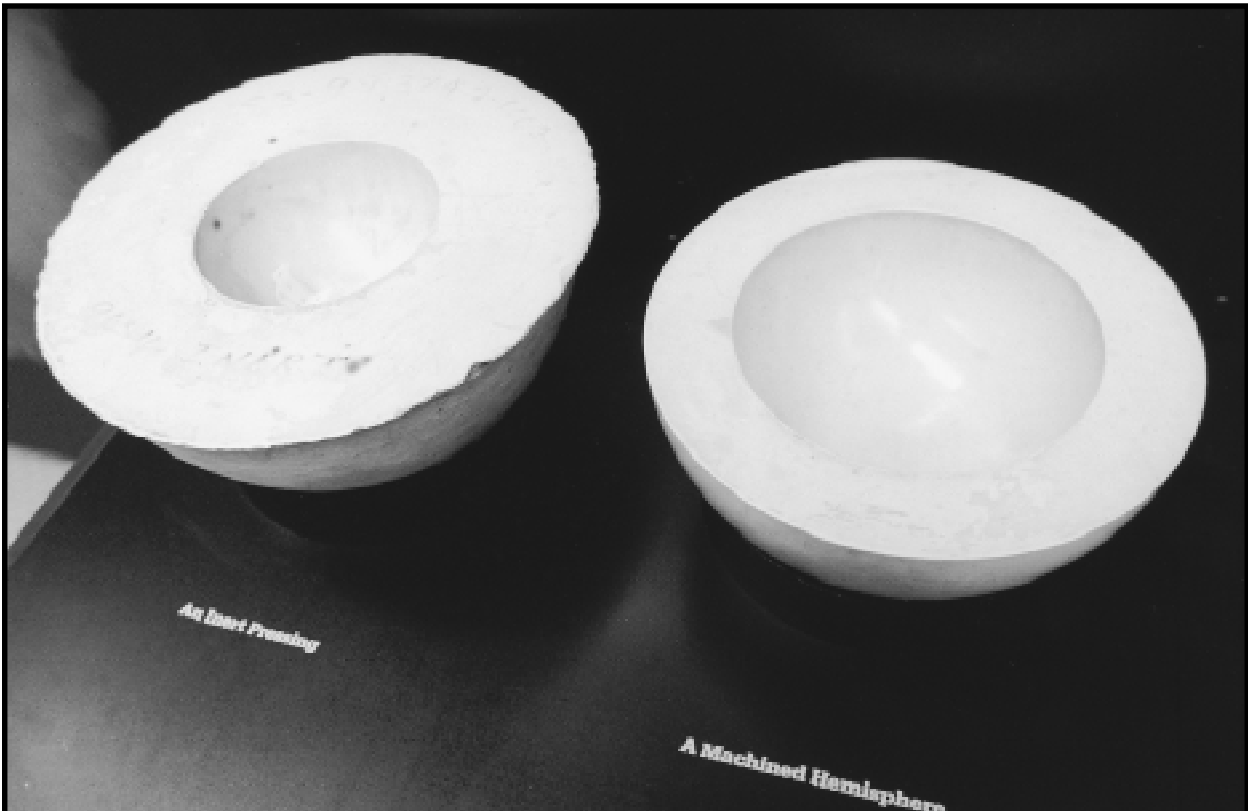
Hemispheres of high explosives configured like the models in this display are used in an implosion bomb to rapidly squeeze a subcritical mass of plutonium into a denser, supercritical state. High explosive components for nuclear weapons were first made at Los Alamos, then at a pilot plant in China Lake, California, then finally at full scale in Burlington, Iowa, and Amarillo, Texas. Bradbury Science Museum, Los Alamos, New Mexico. July 15, 1985.
