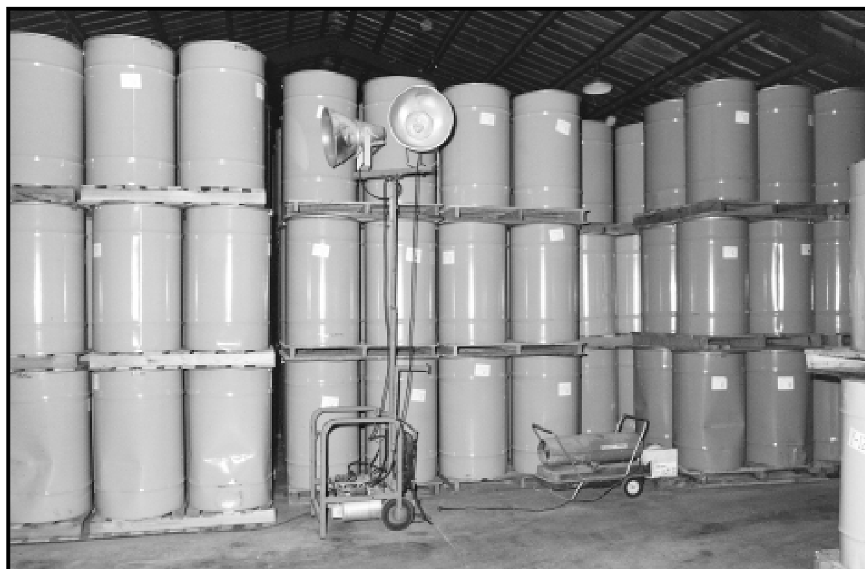
Lithium enrichment "tails," a byproduct of lithium enrichment at Oak Ridge, are stored at the Portsmouth and K-25 plants. The 30.8 million kilograms of lithium tails stored at Portsmouth are stacked from wall to wall and floor to ceiling in a series of "barns." DOE repackaged these materials in the 1980s after their original cardboard containers deteriorated. This lithium was sold to commercial buyers in 1996, and is gradually being shipped off site for use in batteries and other industrial applications. Portsmouth Gaseous Diffusion Plant, Piketon, Ohio. 1986.
