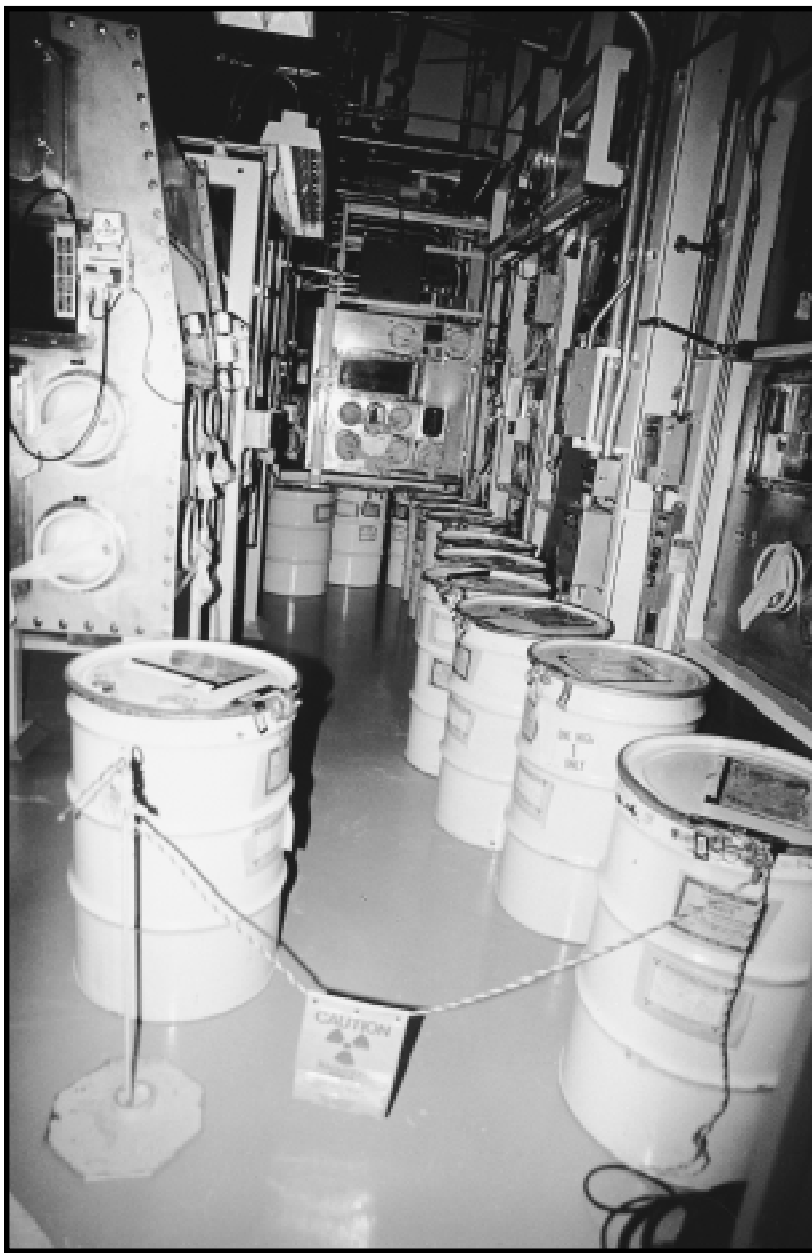
Drums of plutonium-bearing residues at the Rocky Flats Plant contain too much plutonium to be disposed of as transuranic wastes. The residues must be stabilized so that they can be stored safely until final disposition plans have been formulated and carried out. Building 776/777, Rocky Flats Plant, Colorado. December 20, 1993.
