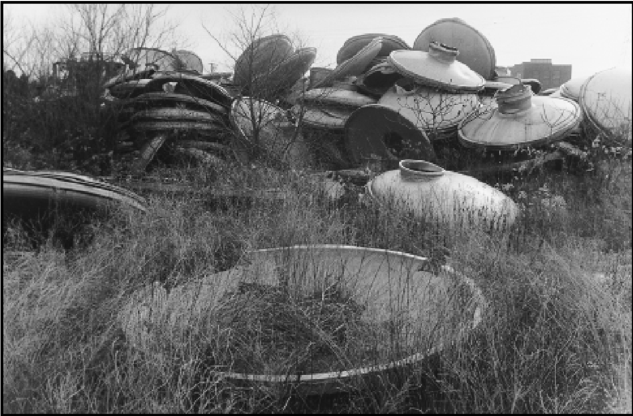
Radioactive scrap metal. Slightly radioactive parts of obsolete uranium enrichment equipment lie in a contaminated scrap-metal yard at Oak Ridge. These 6- and 9-foot wide spun-aluminum disks are categorized as materials in inventory rather than as waste because this metal may be recycled. DOE is recycling some contaminated steel as containers for radioactive waste. Scrap metal constitutes about 20 percent of the Department's Materials in Inventory. K-770 Contaminated Scrap Metal Yard, K-25 Site, Oak Ridge, Tennessee. January 10, 1994.
