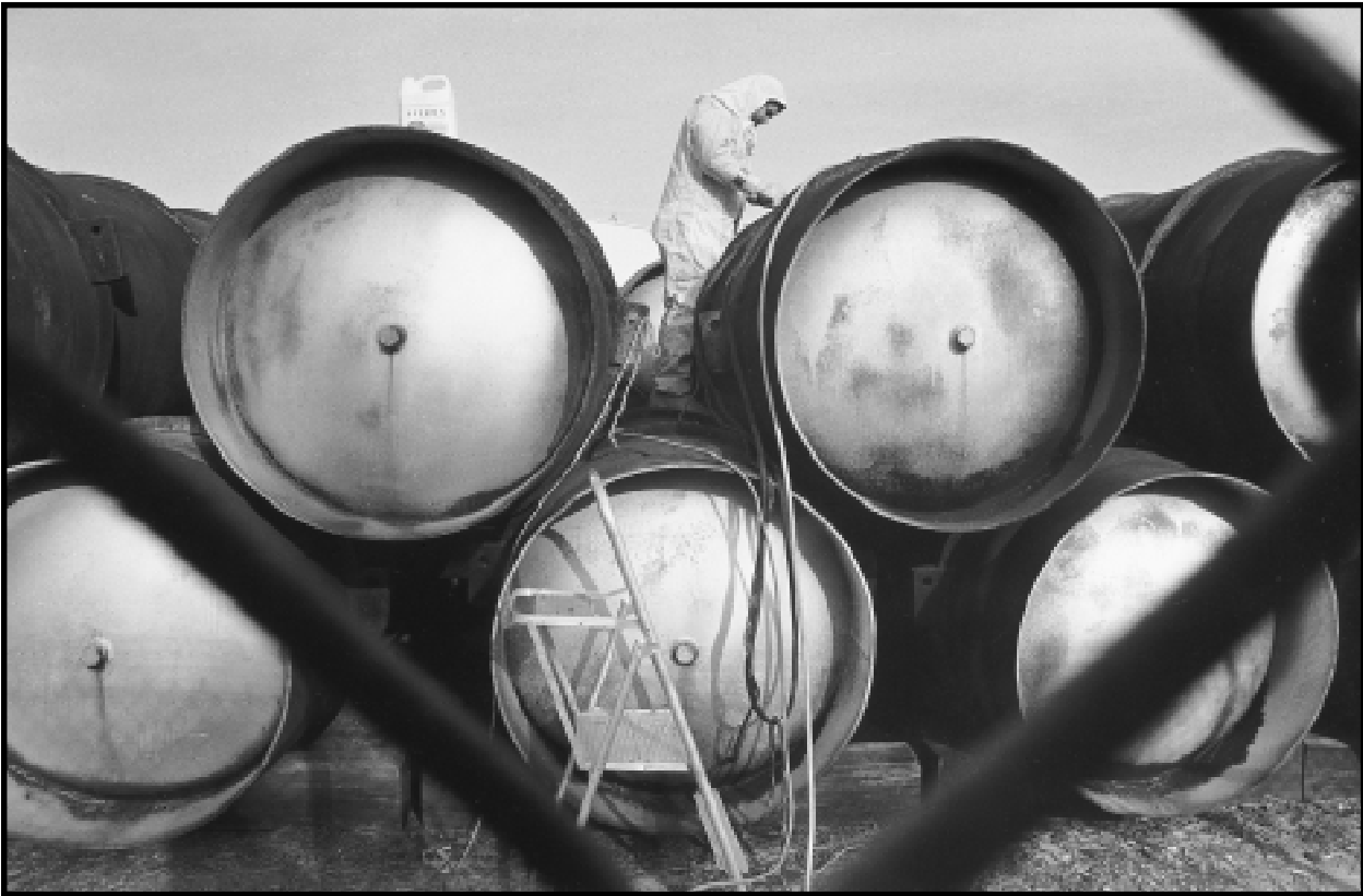
Maintenance of uranium hexafluoride cylinders. An Oak Ridge worker uses ultrasound to evaluate the effects of corrosion on a steel cylinder containing depleted uranium hexafluoride—the material left over from the uranium enrichment process. The Department of Energy owns over 46,000 cylinders of these enrichment “tails,” weighing 10 to 14 tons each. By mass, depleted uranium makes up over 70 percent of the Department’s Materials in Inventory. About one-third of the 585,000 metric tons of this material is a result of nuclear weapons production; most of the rest is from enrichment for commercial nuclear power plant fuel. K-1066-K Cylinder Yard, K-25 Site, Oak Ridge, Tennessee. January 9, 1994.
